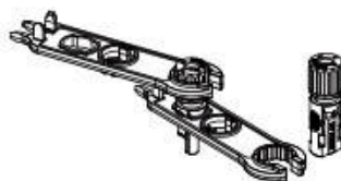
Pic 5.5 connector with cap nut screwed on
