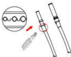
Pic 5.4 Crimp the contact pin to the wire
