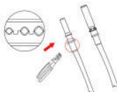
Pic 5.4 Crimp the contact pin to the wire
