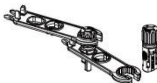
Pic 5.5 connector with cap nut screwed on
